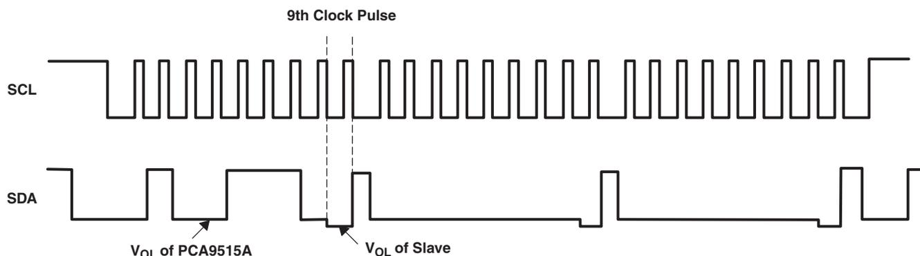
Figure 5. Bus 1 Waveforms
