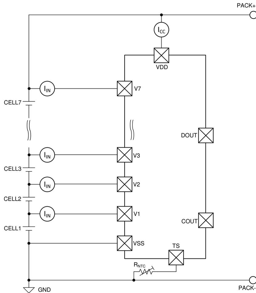
**Figure 10-2. Configuration for IC Current Consumption Test**
