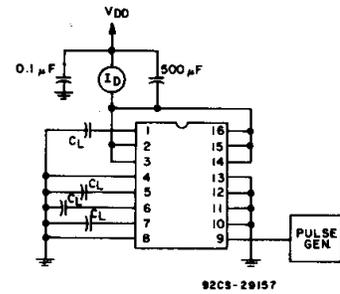
Fig. 9 – Dynamic power dissipation test circuit.
