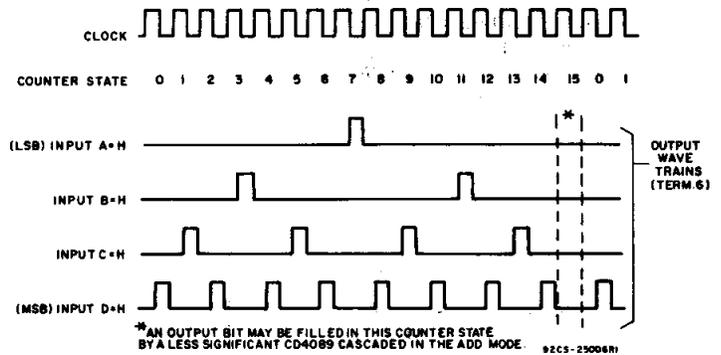
Fig. 15 - Timing diagram.
