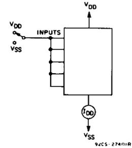
Fig. 10 – Quiescent device current test circuit.
