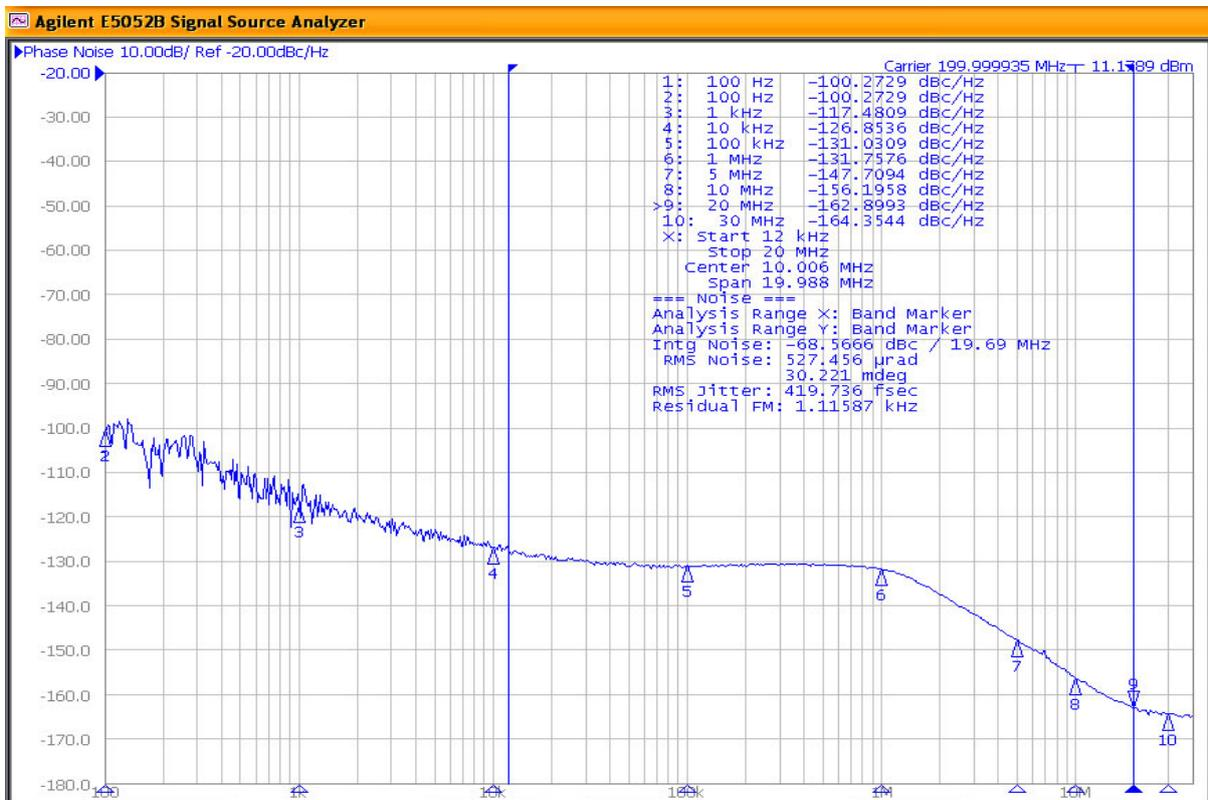
Figure 2. LVC MOS Output 200MHz 12kHz-20MHz 420fs
