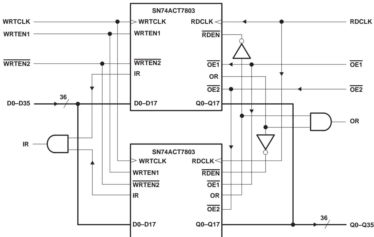
Figure 10. Word-Width Expansion: 512 × 36 Bits
