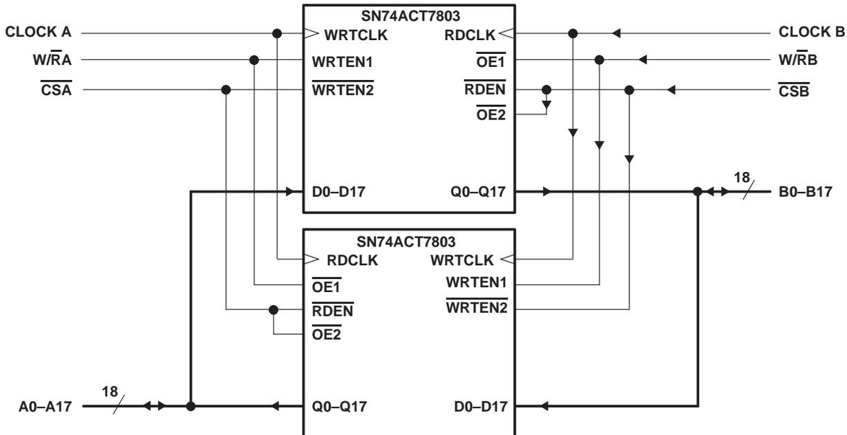
Figure 9. Bidirectional Configuration
