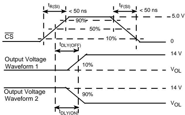
1.  $t_{DLY(ON)}$  and  $t_{DLY(OFF)}$  are turn-ON and turn-OFF propagation delay times.
