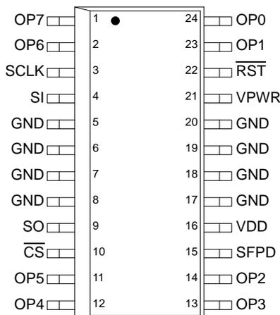
Figure 3. 33291 Pin Connections
