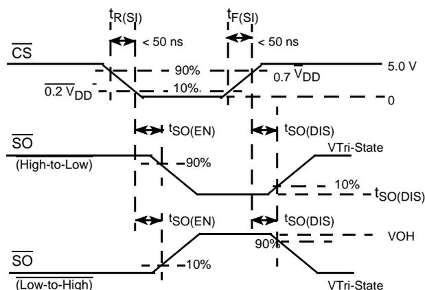
1. SO (high-to-low) waveform is for SO output with internal conditions such that SO output is low except when an output is disabled as a result of detecting a circuit fault with CS in a High Logic state; e.g., open load.
