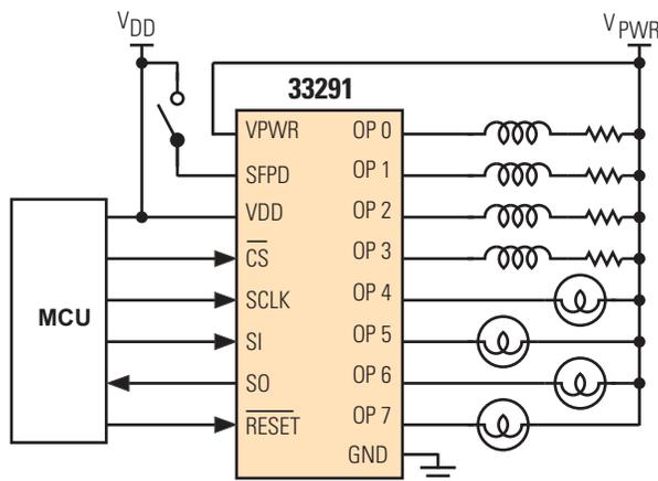
Figure 1. 33291 Simplified Application Schematic
