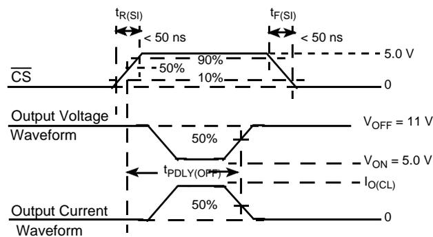
1.  $t_{PDLY(OFF)}$  is the output fault unlatch disable propagation delay time required to correctly report an output fault after  $\overline{CS}$  rises. It represents an output commanded ON while having an existing output short (overcurrent) to supply.
