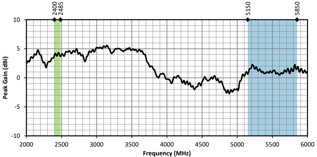
Figure 4. ANT-2/5-HDP-2000 Peak Gain with Frequency Band Highlights
