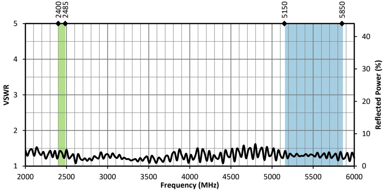
Figure 2. ANT-2/5-HDP-2000 VSWR with Frequency Band Highlights
