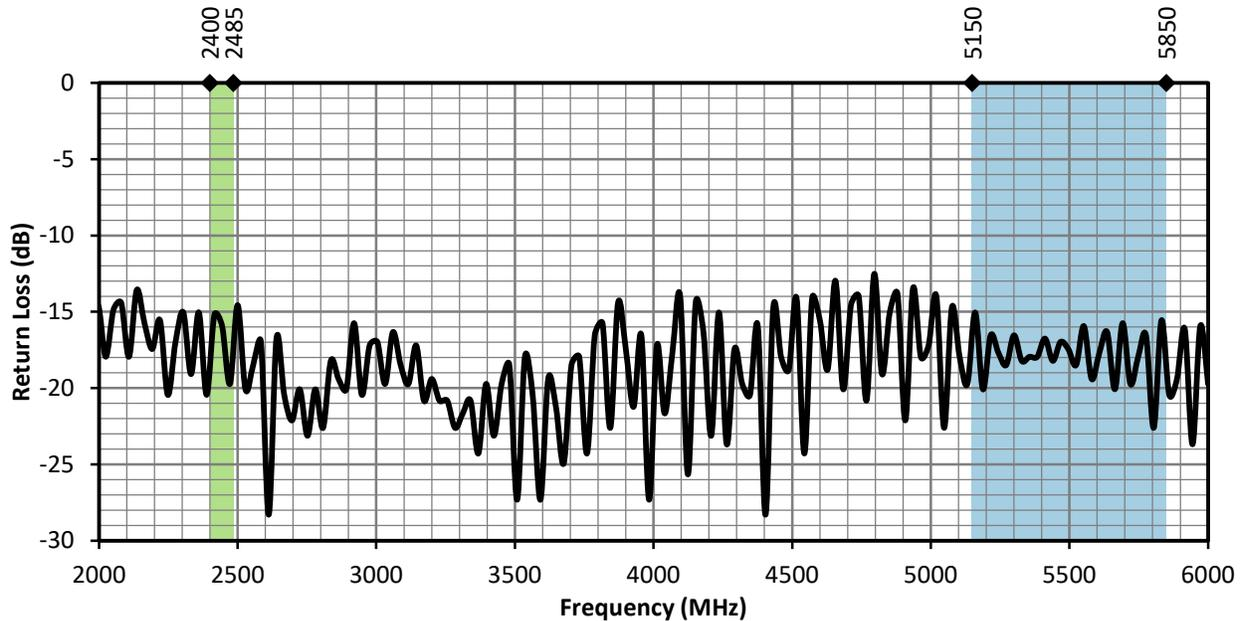
Figure 3. ANT-2/5-HDP-2000 Return Loss with Frequency Band Highlights
