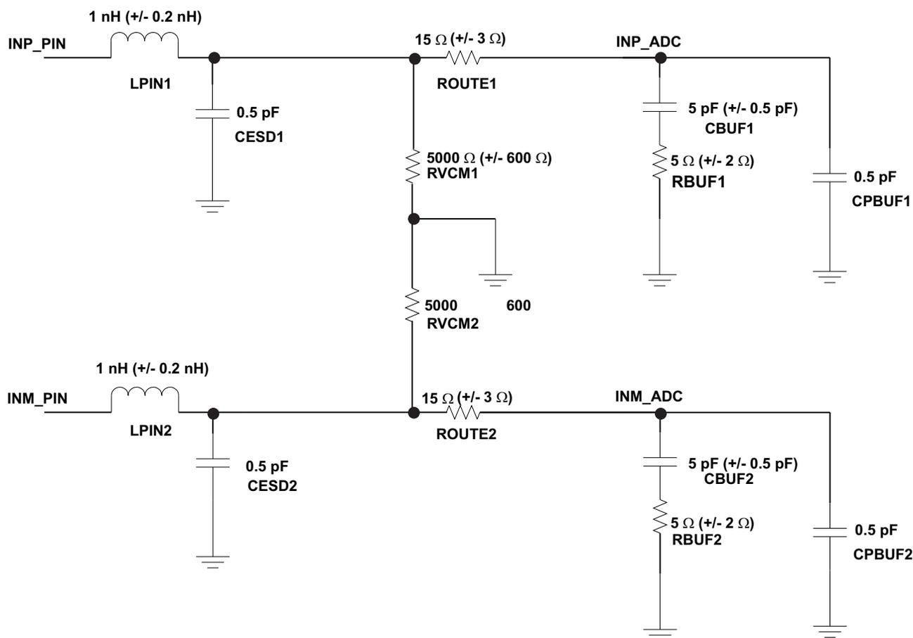
Figure 45. Equivalent Circuit
