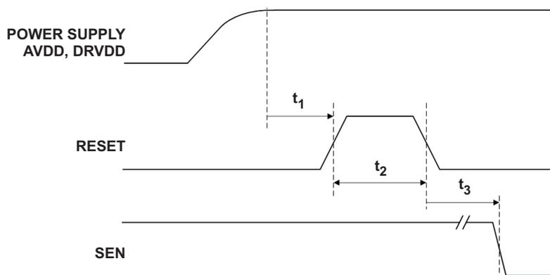
NOTE: A high-going pulse on RESET pin is required in case of initialization through hardware reset.
