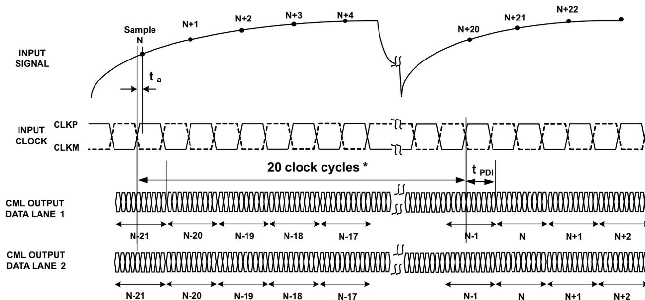
\* This is the ADC latency. At higher sampling frequencies,  $t_{PDI} > 1$  clock cycle. Then, overall latency = ADC latency + 1.
