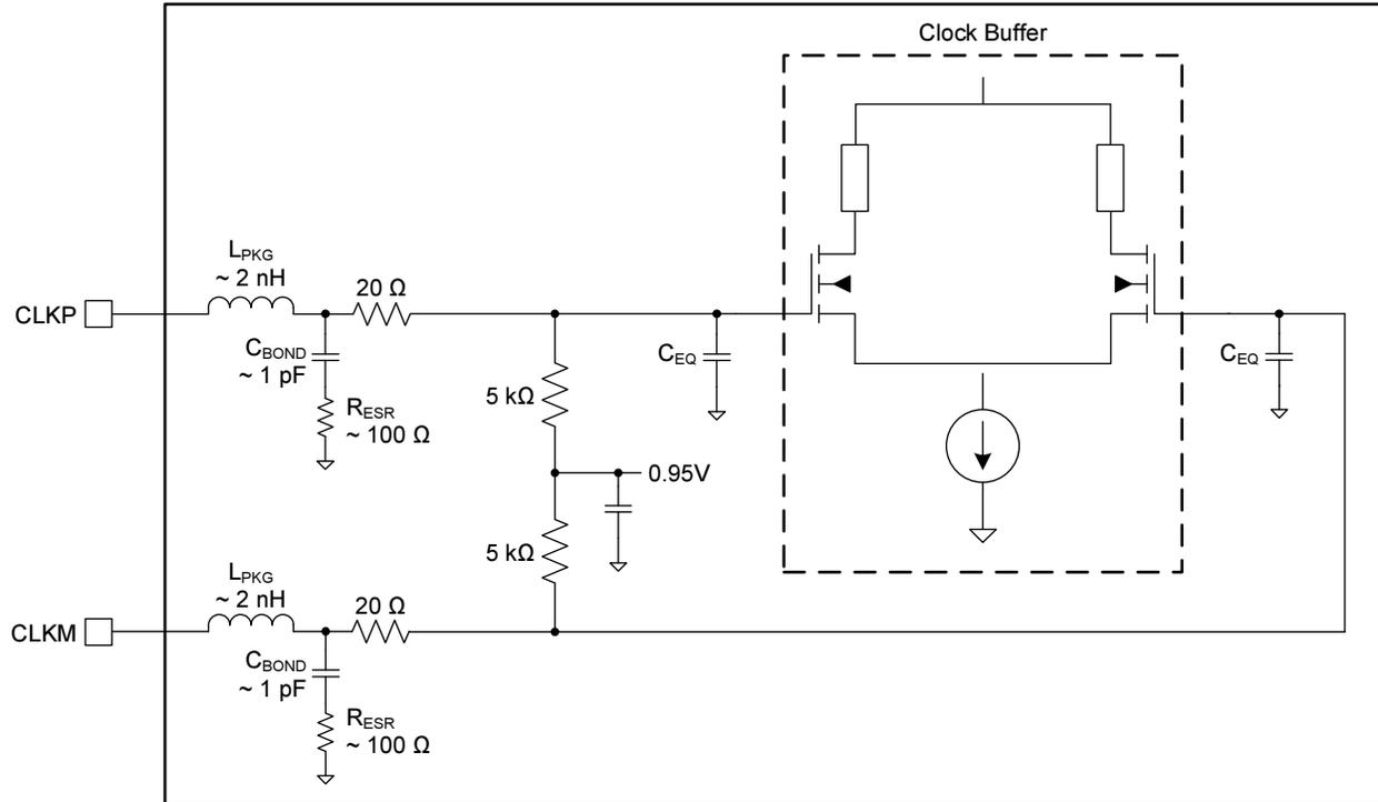
Note:  $C_{EQ}$  is 1pF to 3pF and is the equivalent input capacitance of the clock buffer.
