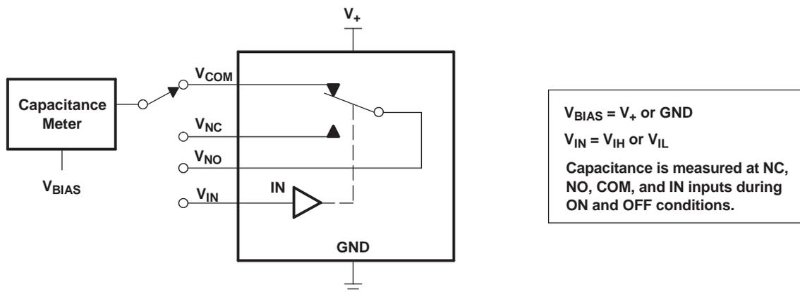
Figure 16. Capacitance ( $C_{IN}$ ,  $C_{COM(ON)}$ ,  $C_{NC(OFF)}$ ,  $C_{NO(OFF)}$ ,  $C_{NC(ON)}$ ,  $C_{NO(ON)}$ )
