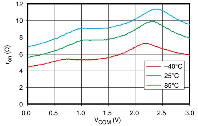
**Figure 2.  $r_{ON}$  vs  $V_{COM}$  ( $V_+ = 3.3$  V)**
