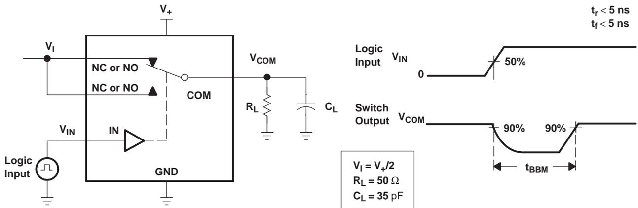
Figure 18. Break-Before-Make (t<sub>BBM</sub>) Time
