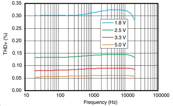
**Figure 10. Total Harmonic Distortion (THD) vs Frequency**
