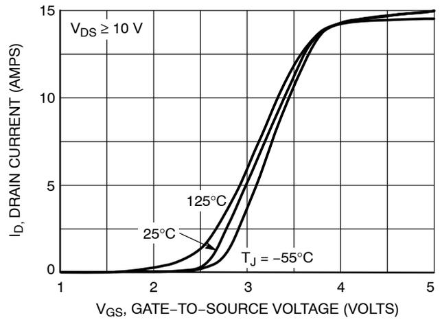
Figure 2. Transfer Characteristics
