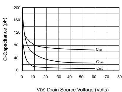
**Capacitance v drain-source voltage**
