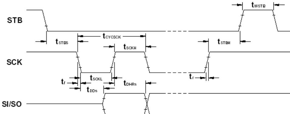
Figure 7. Synchronous Serial Interface Read Cycle Timing
