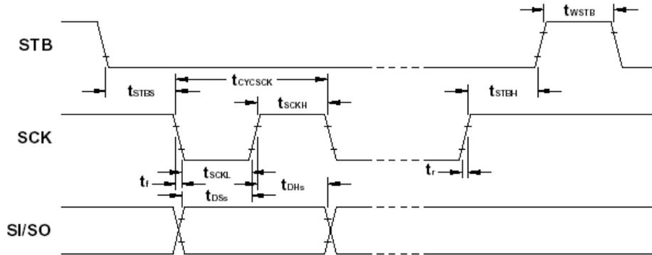
Figure 6. Synchronous Serial Interface Write Cycle Timing
