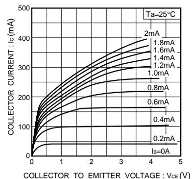
Fig.3 Grounded emitter output characteristics ( II )
