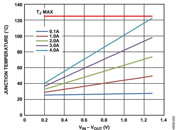
Figure 52. 100 mm<sup>2</sup> of PCB Copper,  $T_B = 25^\circ\text{C}$
