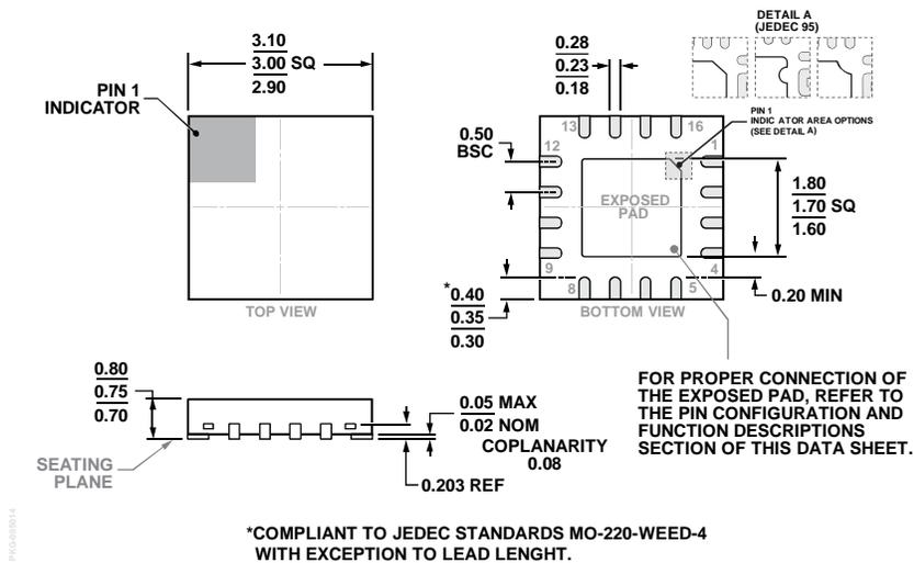
Figure 60. 16-Lead Lead Frame Chip Scale Package [LFCS]
