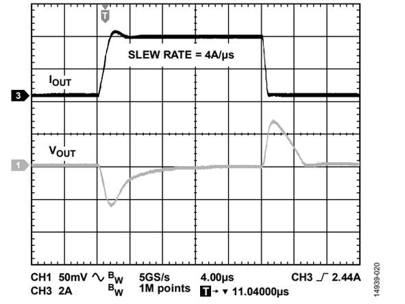
Figure 20. Load Transient Response,  $C_{OUT} = 22\mu F$ ,  $V_{IN} = 1.8V$ ,  $V_{OUT} = 1.3V$
