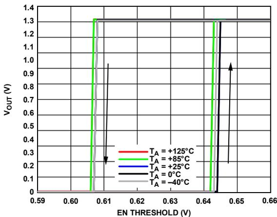
Figure 43. Output Voltage vs. EN Threshold,  $V_{OUT} = 1.3 V$
