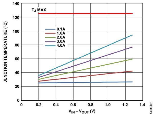
Figure 51. 500 mm<sup>2</sup> of PCB Copper,  $T_B = 25^\circ\text{C}$
