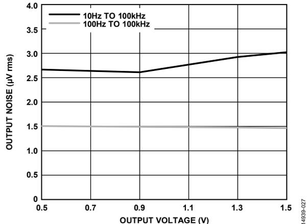
Figure 27. Output Noise vs. Output Voltage ( $V_{OUT}$ )
