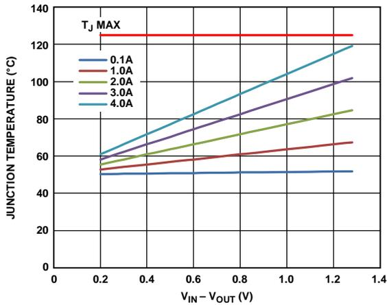
Figure 54. 500 mm<sup>2</sup> of PCB Copper,  $T_B = 50^\circ\text{C}$ , LFCSP
