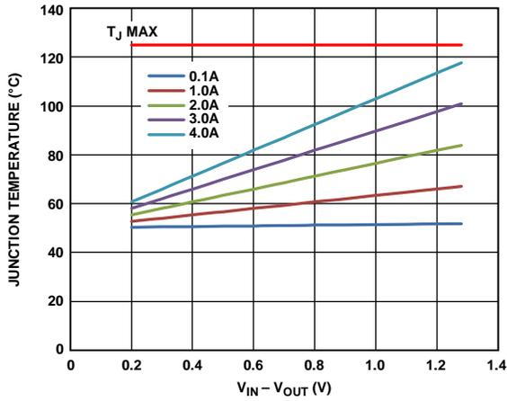
Figure 53. 1000 mm<sup>2</sup> of PCB Copper,  $T_B = 50^\circ\text{C}$ , LFCSP
