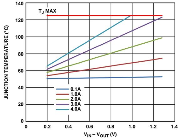
Figure 55. 100 mm<sup>2</sup> of PCB Copper,  $T_B = 50^\circ\text{C}$ , LFCSP
