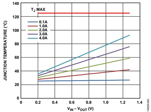
Figure 50. 1000 mm<sup>2</sup> of PCB Copper,  $T_B = 25^\circ\text{C}$
