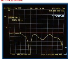
Fig 2.0 RF Coupler Insertion Loss S21 (dB) \*
