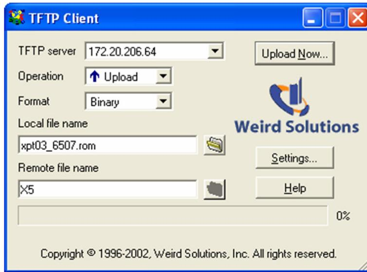
6. Click the **Upload Now** button to transfer the file to the unit. The unit performs a power reset after the firmware has been loaded and stored.
