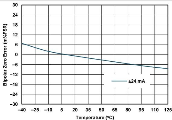
Figure 13. IOUT Bipolar Zero Error vs Temperature
