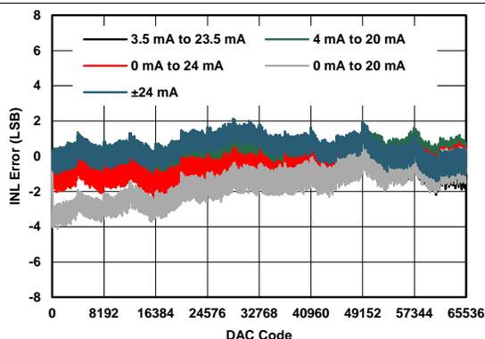
Figure 3. IOUT Linearity Error vs Digital Input Code
