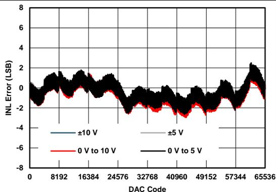
Figure 44. VOUT Linearity Error vs Digital Input Code
