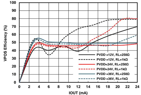
Figure 89. VPOS Efficiency (IOOUT Mode) vs Load Current
