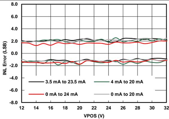
Figure 15. IOU Linearity Error vs Power Supplies
