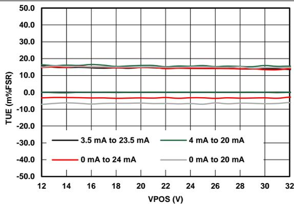
Figure 19. IOU Total Unadjusted Error vs Power Supplies
