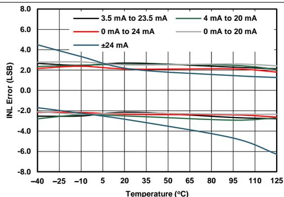
Figure 6. IOUT Linearity Error vs Temperature
