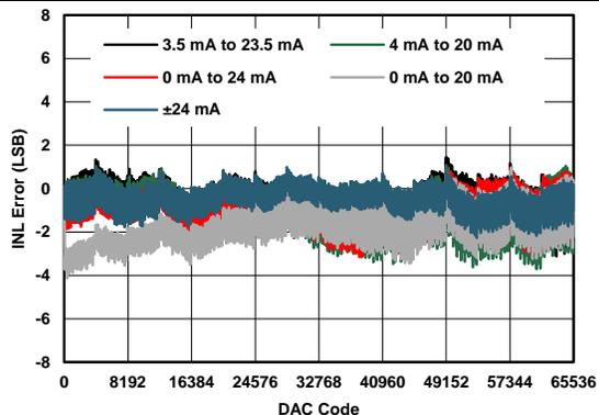
Figure 35. IOUT Linearity Error vs Digital Input Code
