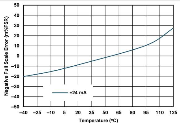
Figure 14. IOUT Negative Full Scale Error vs Temperature
