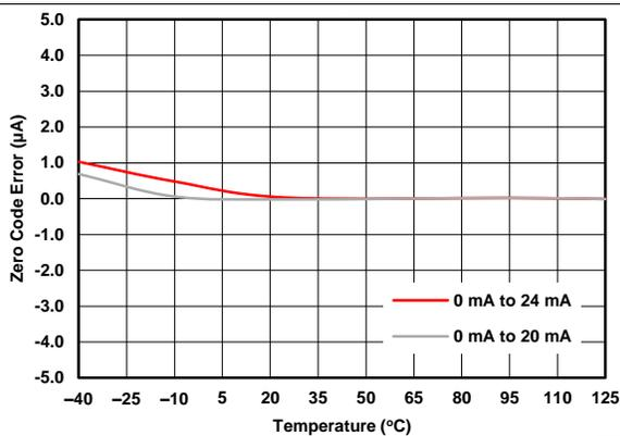
Figure 11. IOUT Zero Code Error vs Temperature
