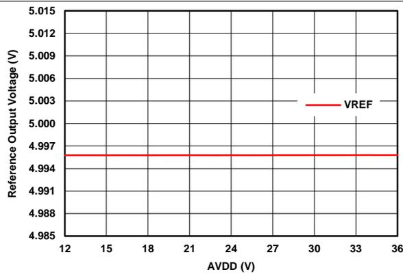
Figure 78. Internal Reference Voltage vs Power Supply
