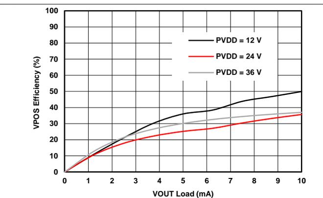
Figure 95. VPOS Efficiency (VOUT Mode) vs Load Current
