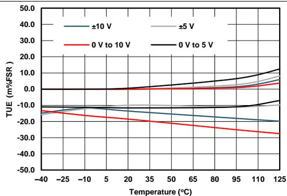
Figure 49. VOUT Total Unadjusted Error vs Temperature
