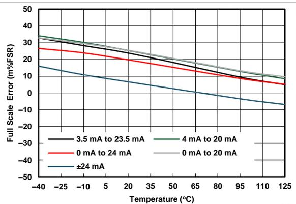
Figure 12. IOUT Full Scale Error vs Temperature
