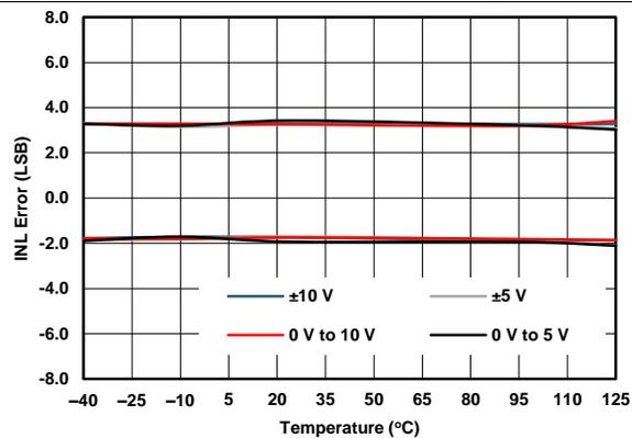
Figure 47. VOUT Linearity Error vs Temperature
