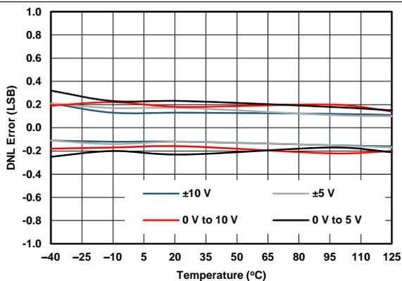
Figure 48. VOUT Differential Linearity Error vs Temperature
