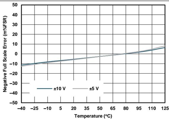
Figure 54. VOUT Negative Full Scale Error vs Temperature
