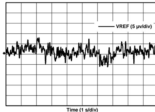
Figure 80. Internal Reference Noise, 0.1 Hz to 10 Hz
