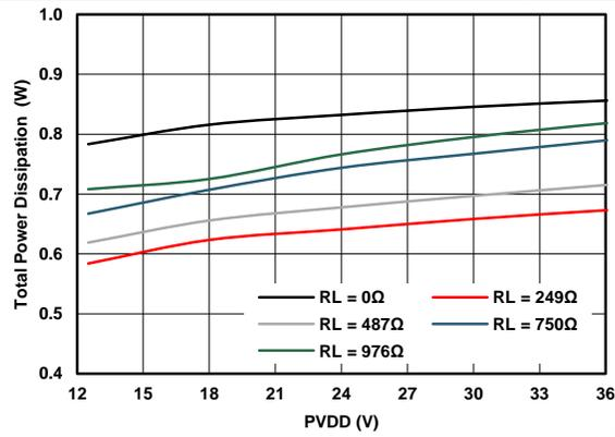
**Figure 134. Total On-Board Power Dissipation vs Supply**
