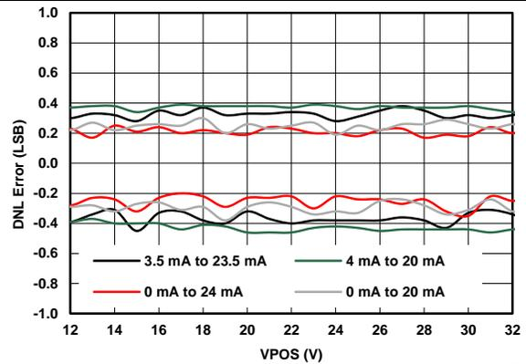
Figure 16. IOU Differential Linearity Error vs Power Supplies
