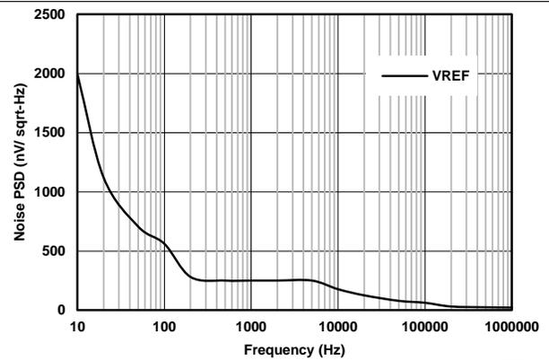
Figure 79. Internal Reference Noise Density vs Frequency
