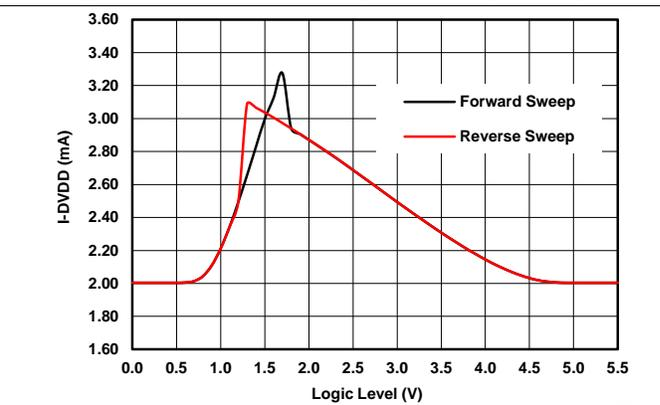
Figure 99. Power Supply Current (DVDD) vs Input Logic Level
