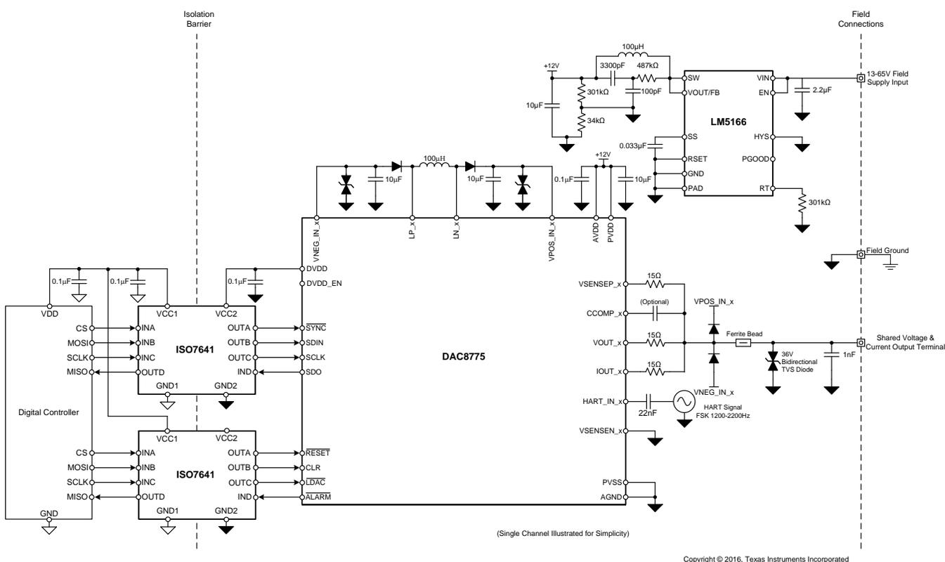
Figure 130. DAC8775 in Quad-Channel PLC AO Module
