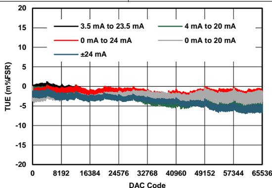
Figure 37. IOUT Total Unadjusted Error vs Digital Input Code
