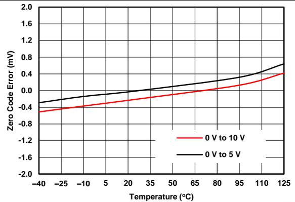
Figure 51. VOUT Zero Code Error vs Temperature
