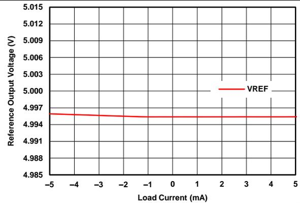
Figure 77. Internal Reference Voltage vs Load Current
