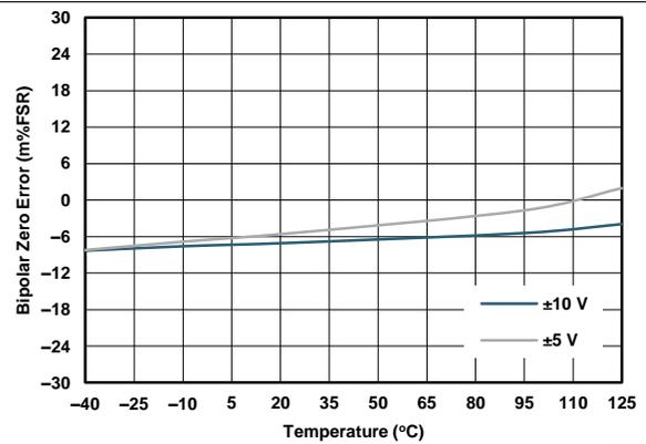
Figure 53. VOUT Bipolar Zero Error vs Temperature
