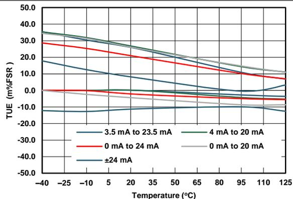
Figure 8. IOUT Total Unadjusted Error vs Temperature
