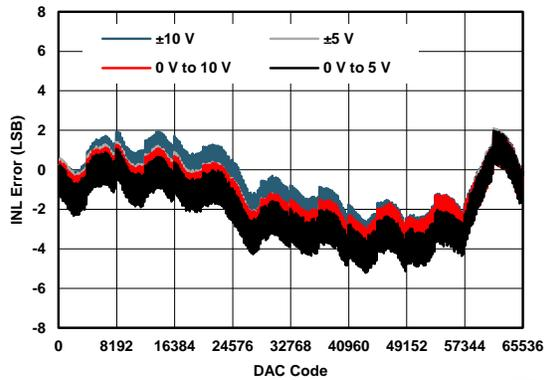
Figure 71. VOUT Linearity Error vs Digital Input Code
