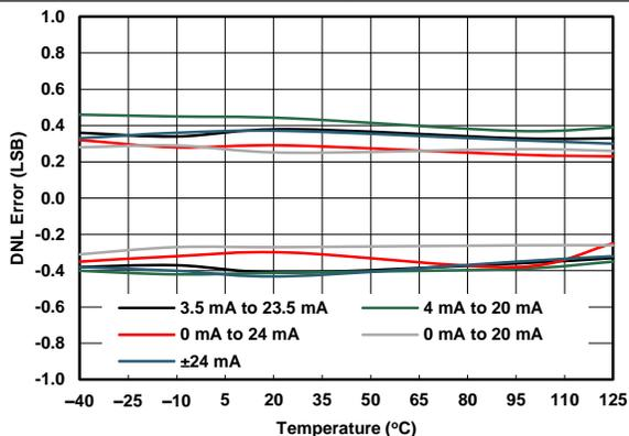
Figure 7. IOUT Differential Linearity Error vs Temperature
