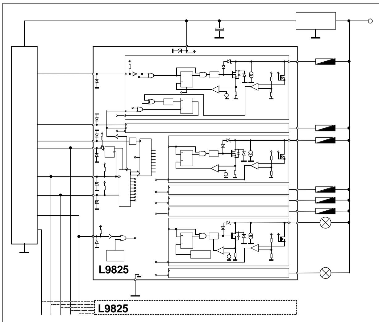
For higher current driving capability two outputs of the same kind can be paralleled. In this case the maximum flyback energy should not exceed the limit value for single output.
