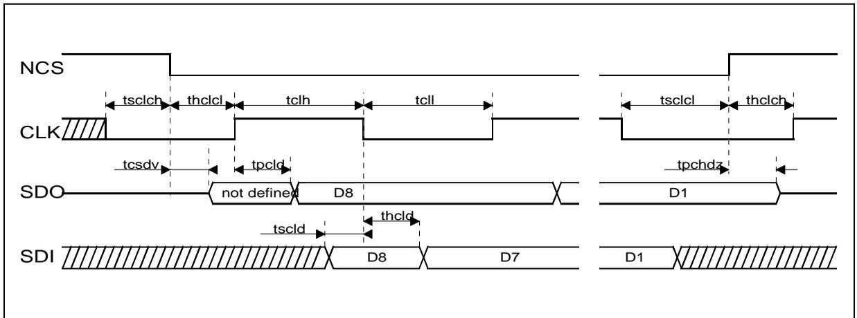
The SPI register data are transferred to the output latch at rising NCS edge. The digital filter between NCS and the output latch ensures that the data are transferred only after 8 CLK cycles or multiple of 8 CLK cycles since the last NCS falling edge. The NCS changes only at low CLK.
