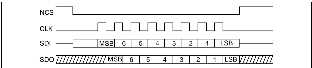
**Figure 4. The Structure of the Outputs Status Register**
