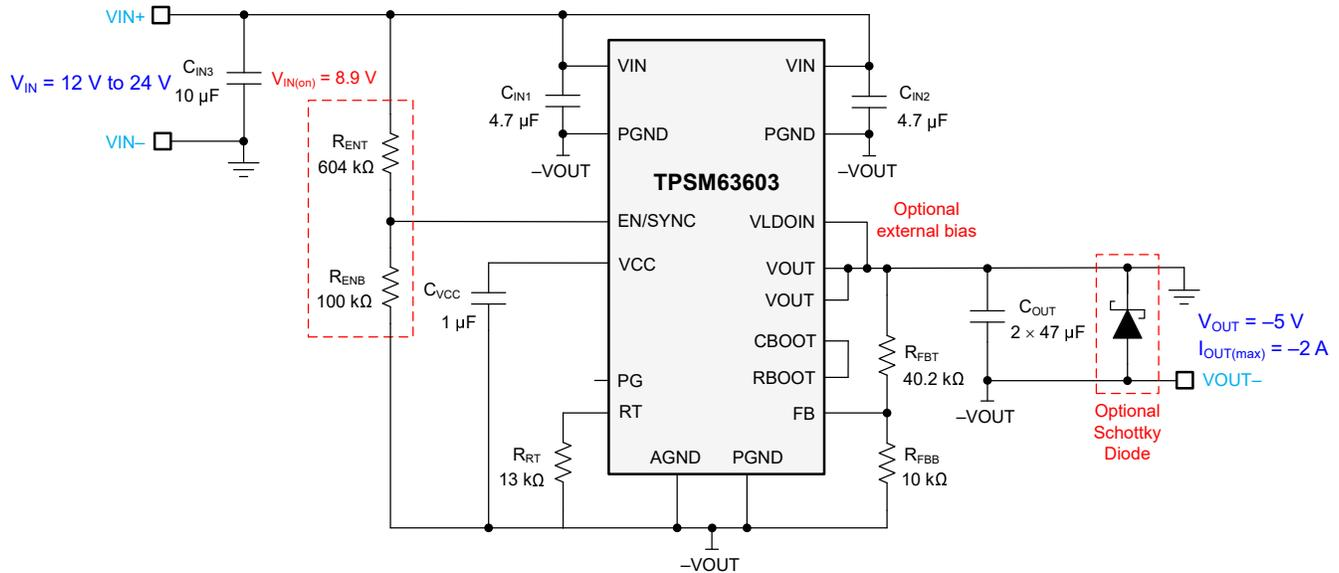
Figure 8-12. Circuit Schematic
