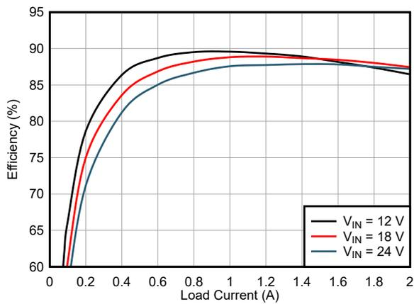
**Figure 8-13. Efficiency Curves**
