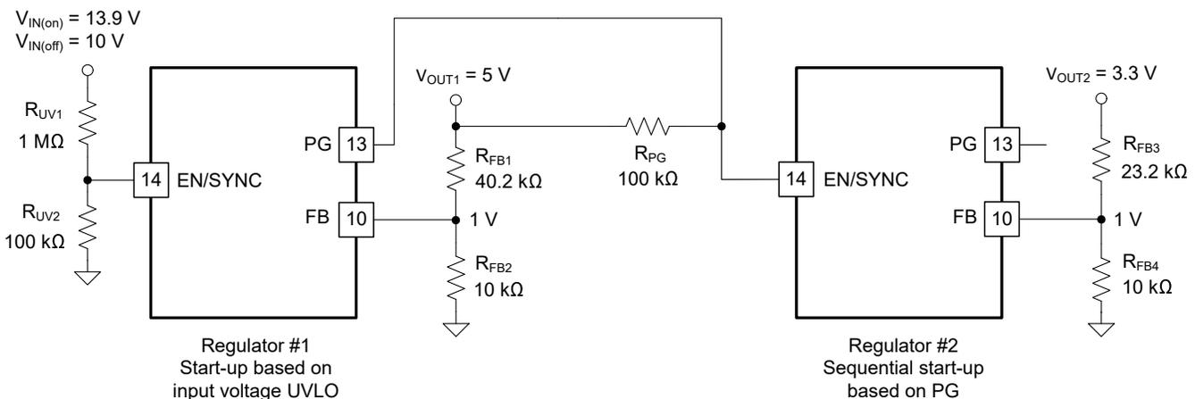
**Figure 7-6. TPSM63603 Sequencing Implementation Using PG and EN/SYNC**
