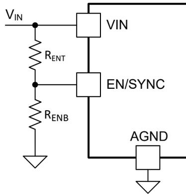
**Figure 7-3. VIN UVLO Using the EN/SYNC Pin**
