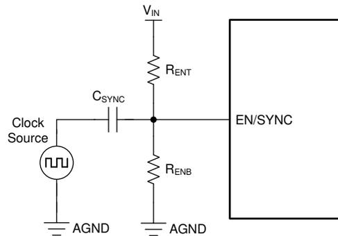
**Figure 7-4. Typical Synchronization Using the EN/SYNC Pin**
