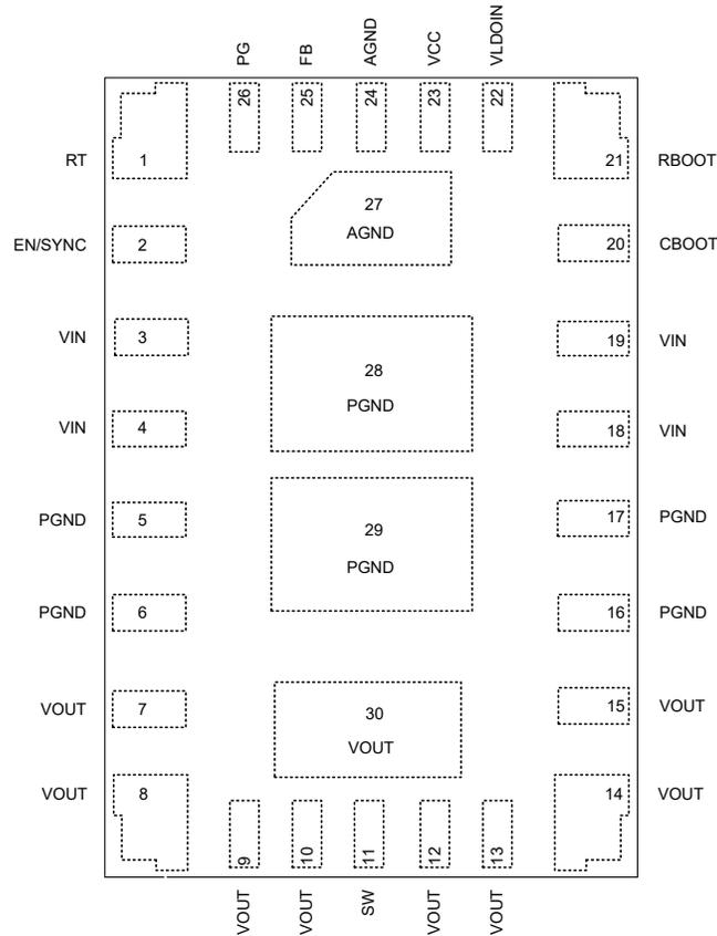
**Figure 5-1. 30-Pin QFN, RDH Package (Top View)**
