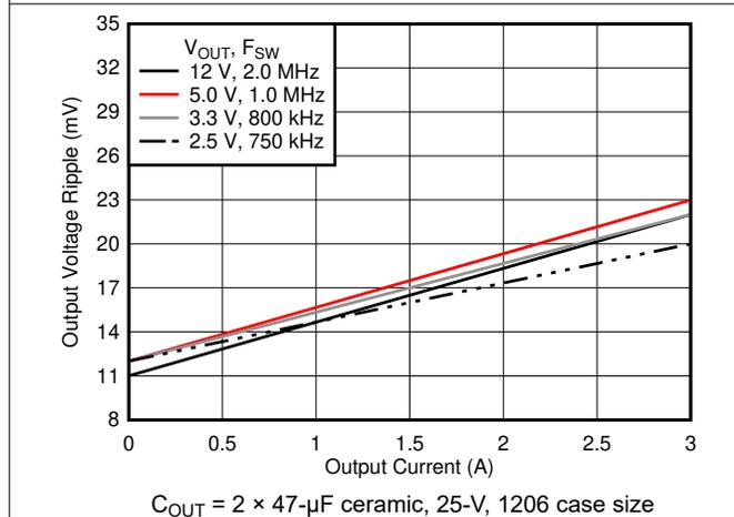
**Figure 6-15. Output Voltage Ripple**
