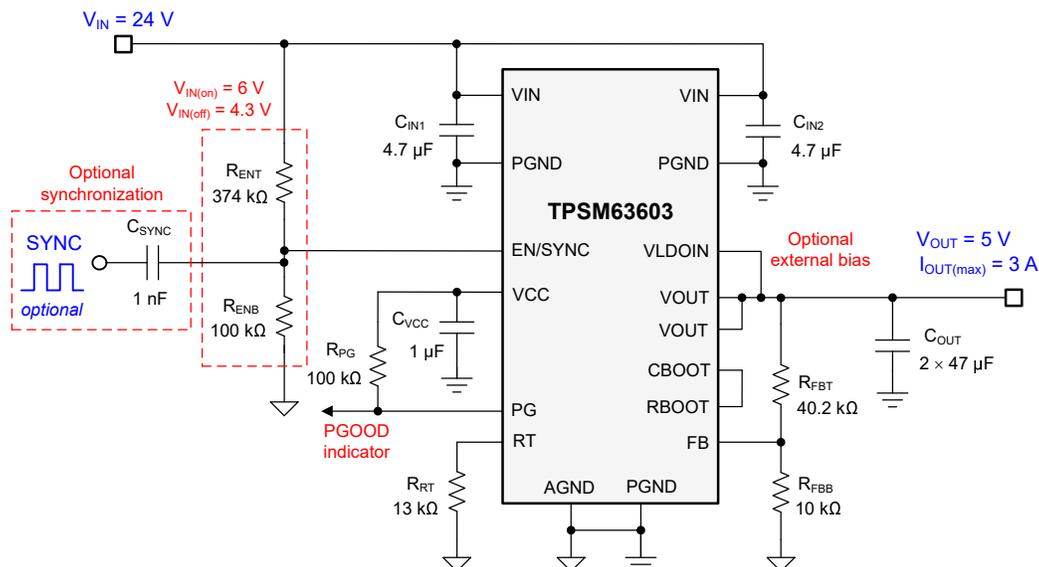
Figure 8-1. Circuit Schematic
