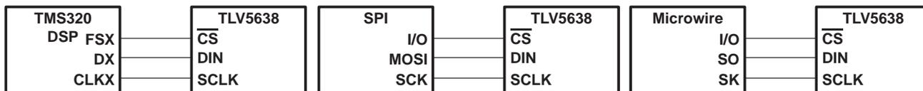
**Figure 13. Three-Wire Interface**
