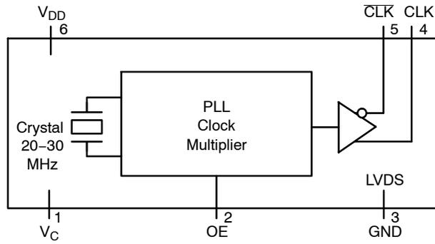
Figure 1. Simplified Logic Diagram
