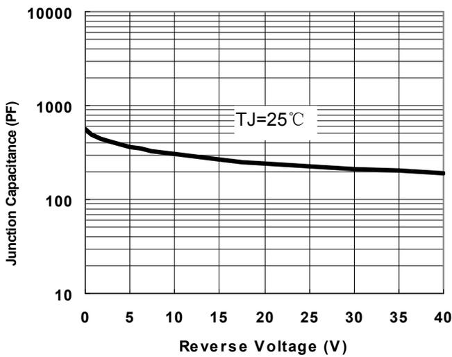
Fig.1-Typical Junction Capacitance
