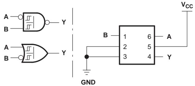
Figure 4. 2-Input NAND Gate With One Inverted Input
