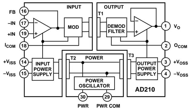
mode voltage isolation between any two ports. Low input capacitance of 5 pF results in a 120 dB CMR at a gain of 100, and a low leakage current (2  $\mu$ A rms max @ 240 V rms, 60 Hz).
