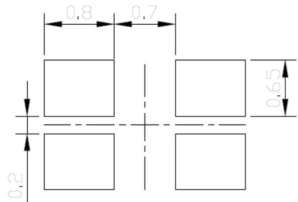
Figure 1. IN-S66TCTRGBE Solder Pattern
