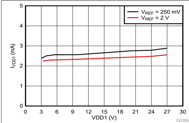
Figure 6-29. High-Side Supply Current vs Supply Voltage
