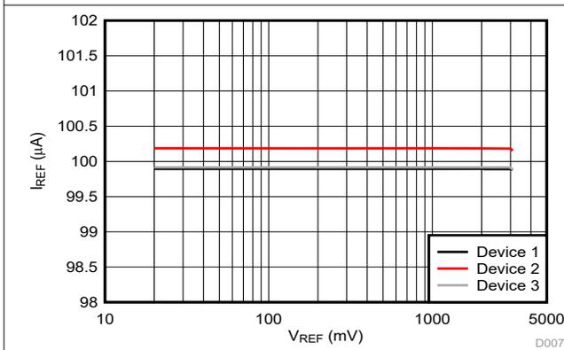
Figure 6-27. Reference Current vs Reference Voltage
