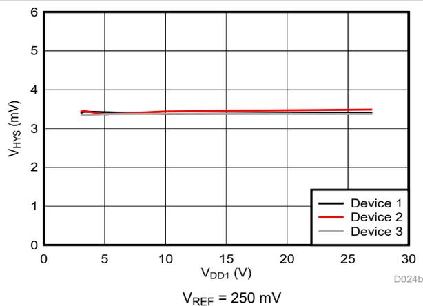
Figure 6-15. Trip Threshold Hysteresis vs Supply Voltage
