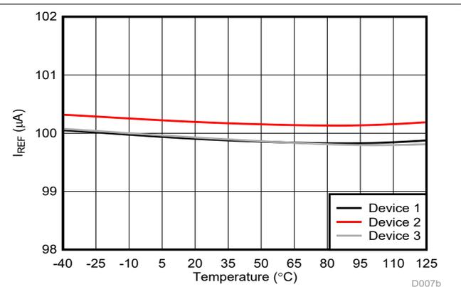
Figure 6-28. Reference Current vs Temperature
