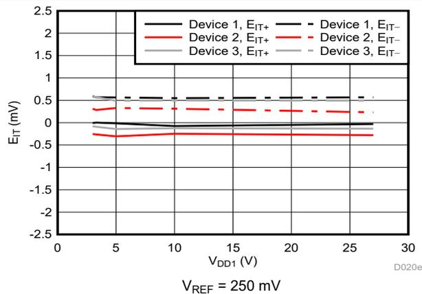
Figure 6-13. Trip Threshold Error vs Supply Voltage
