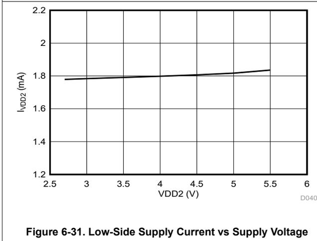
Figure 6-31. Low-Side Supply Current vs Supply Voltage
