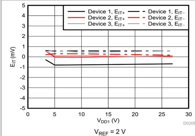
Figure 6-19. Trip Threshold Error vs Supply Voltage
