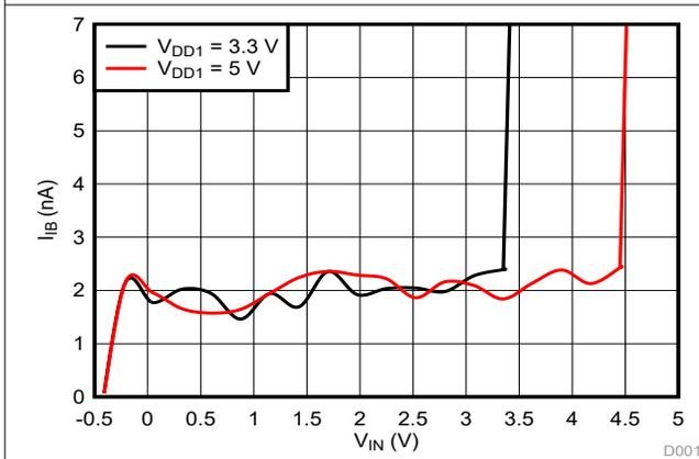
Figure 6-25. Input Bias Current vs Input Voltage
