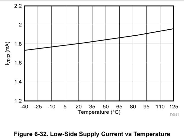
Figure 6-32. Low-Side Supply Current vs Temperature
