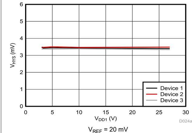
Figure 6-9. Trip Threshold Hysteresis vs Supply Voltage
