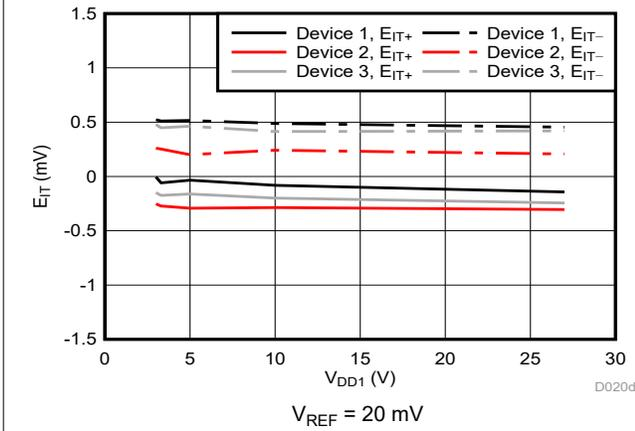
Figure 6-7. Trip Threshold Error vs Supply Voltage
