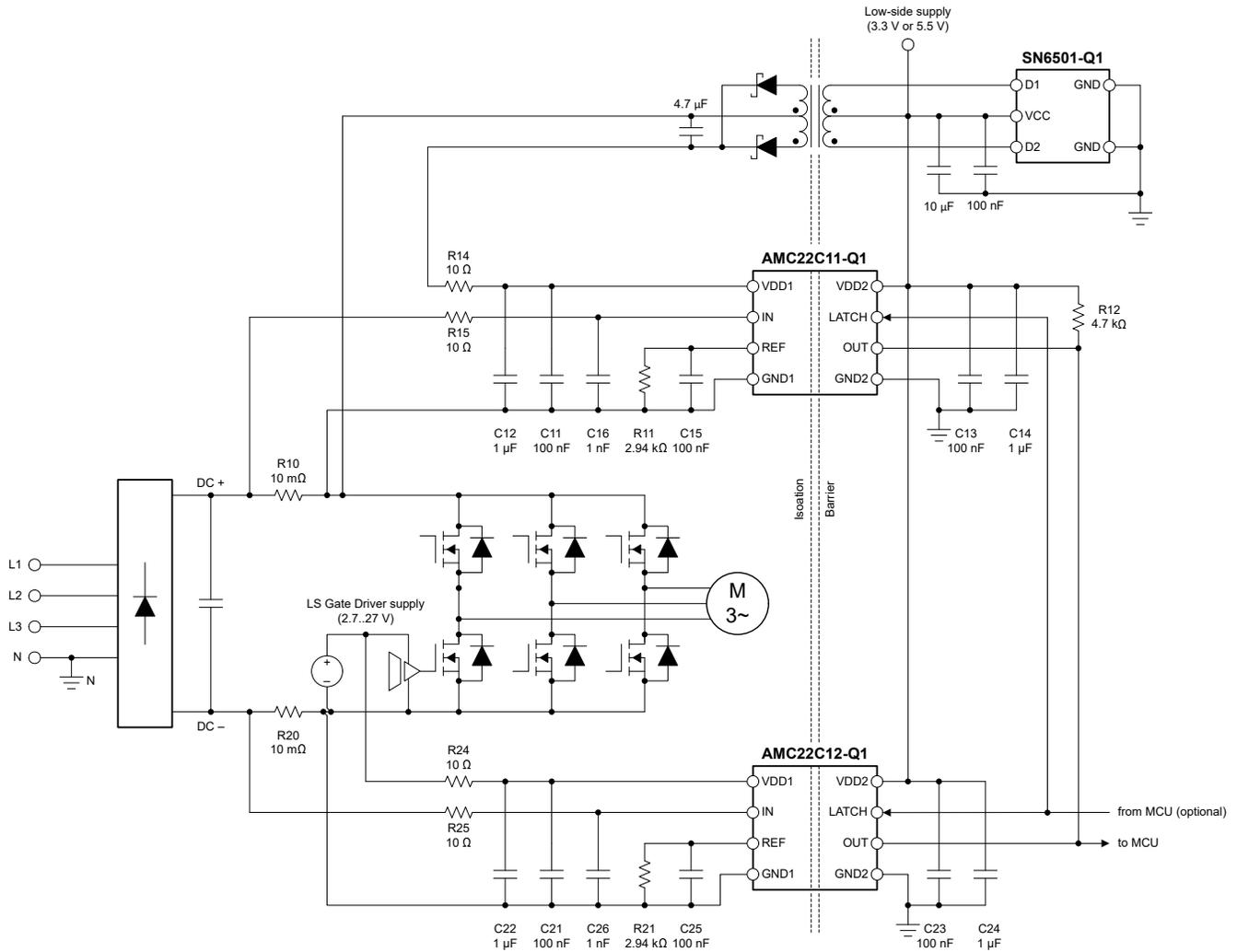
Figure 8-1. Using the AMC22C11-Q1 for DC+ Overcurrent Detection
