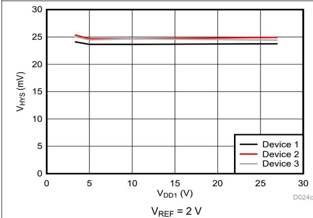
Figure 6-21. Trip Threshold Hysteresis vs Supply Voltage
