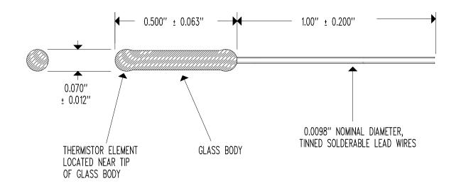
RESISTANCE @  $+25^{\circ}$ C = 1,200  $\pm$  5% RESISTANCE/TEMPERATURE CURVE = "E" BETA " $\beta$ " (+25 TO +85°C) = 3,348°K NOMINAL TEMPERATURE COEFFICIENT @  $+25^{\circ}$ C = -3.67%/°C NOMINAL TEMPERATURE RATING = -50 TO  $+300^{\circ}$ C
