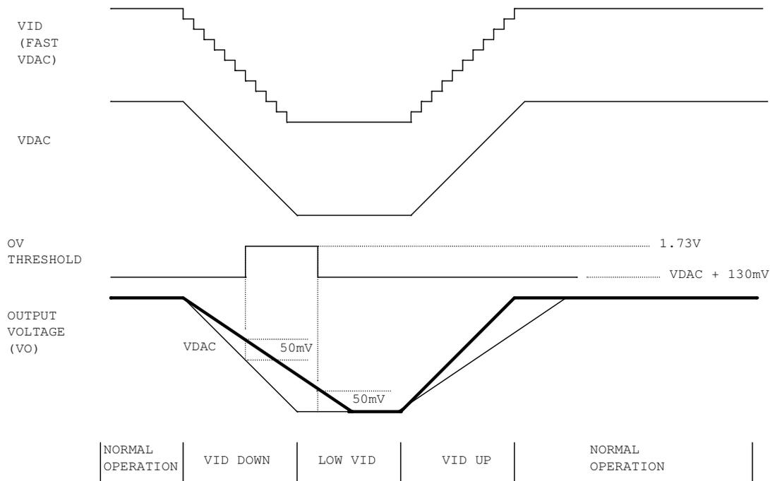
Figure 19 - Over-voltage protection during dynamic VID
