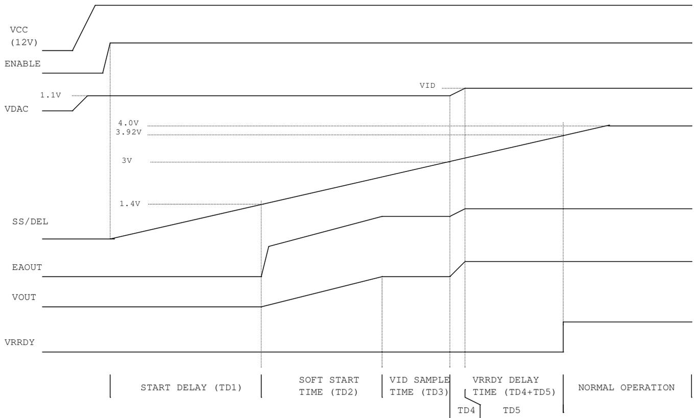
Figure 11 - Start-up sequence of converter with boot voltage
