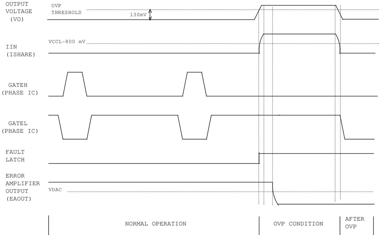
Figure 15 - Over-voltage protection during normal operation
