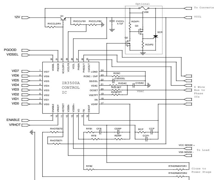
Figure 1 – Application Circuit
