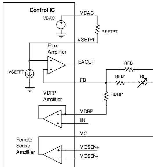
Figure 10 - Temperature compensation of inductor DCR
