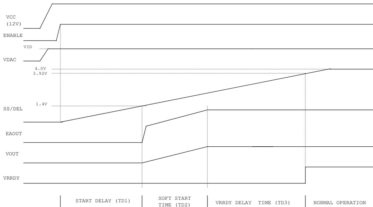
Figure 12 - Start-up sequence of converter without boot voltage
