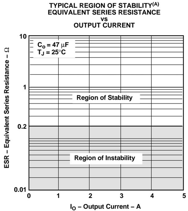
A. Equivalent series resistance (ESR) refers to the total series resistance, including the ESR of the capacitor, any series resistance added externally, and PWB trace resistance to  $C_O$ .
