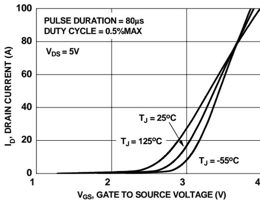
Figure 5. Transfer Characteristics
