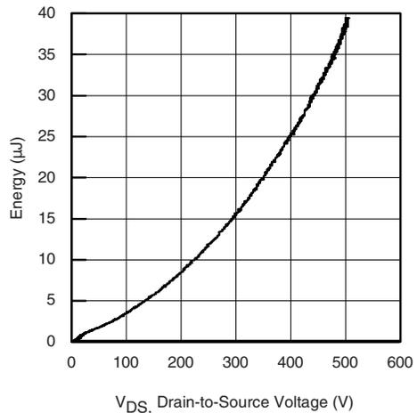
**Fig. 6 - Typical Output Capacitance Stored Energy vs. VDS**
