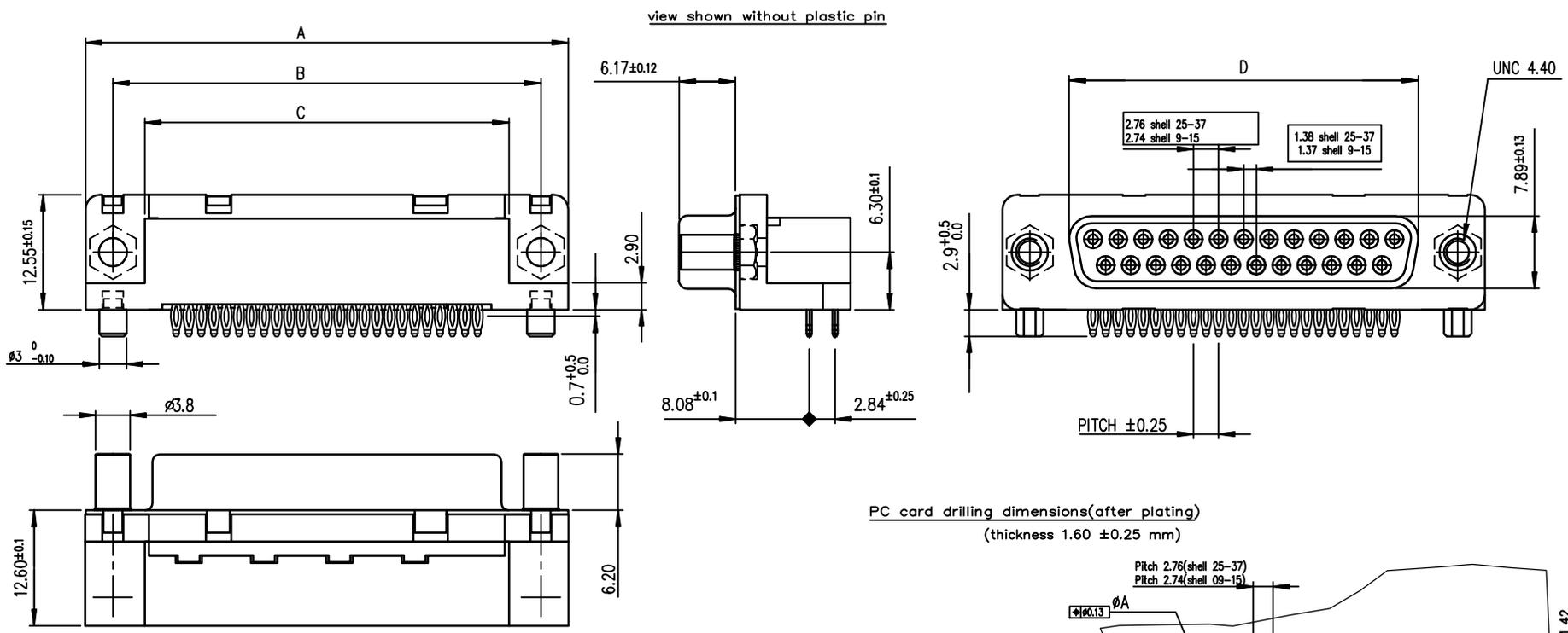
PC card drilling dimensions(after plating)
