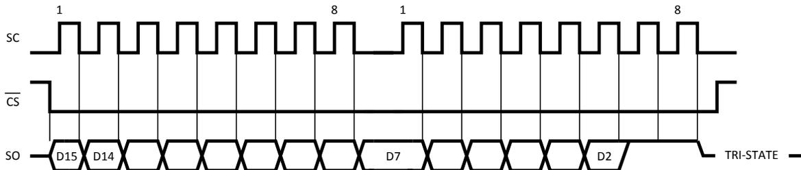
Figure 11. Reading Continuous Conversion - Two Eight-Bit Frames
