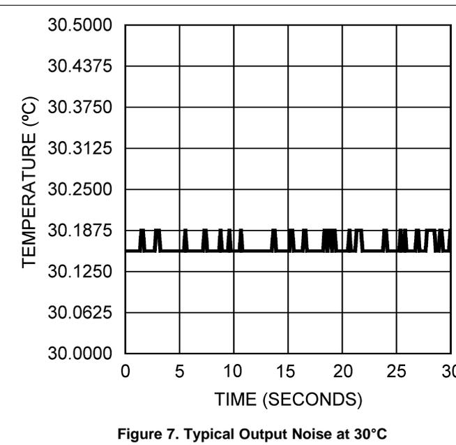
Figure 7. Typical Output Noise at 30°C
