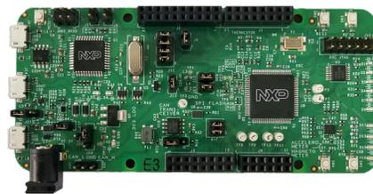
The MC56F83000-EVK is an ultra-low-cost development platform for the MC56F83xxx DSC family allowing rapid prototyping and application development.
