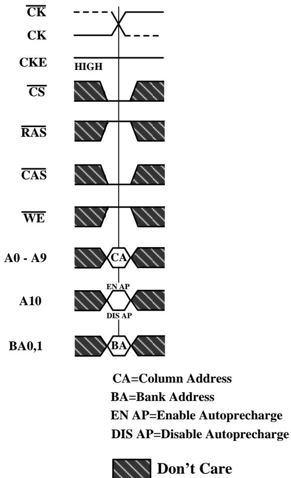
**Figure 7. Read Burst Required CAS Latencies (CL=2)**
