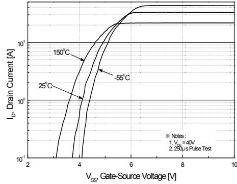
**Figure 2. Transfer Characteristics**
