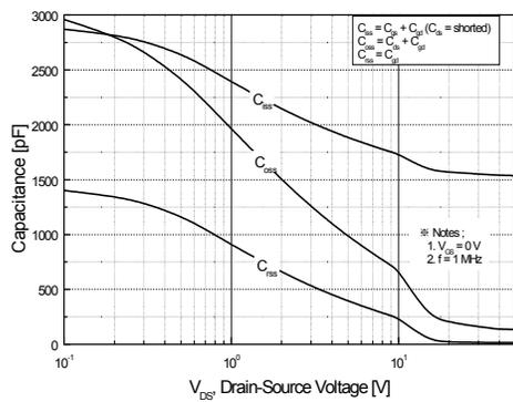
**Figure 5. Capacitance Characteristics**
