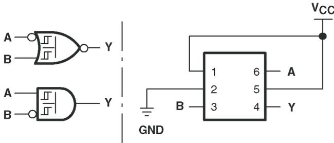
Figure 3. 2-Input NOR Gate With One Inverted Input
