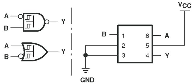
Figure 4. 2-Input NAND Gate With One Inverted Input
