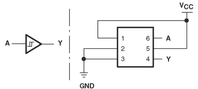
Figure 6. Noninverted Buffer
