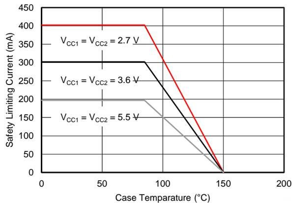
Figure 16.  $\theta_{JC}$  Thermal Derating Curve per VDE
