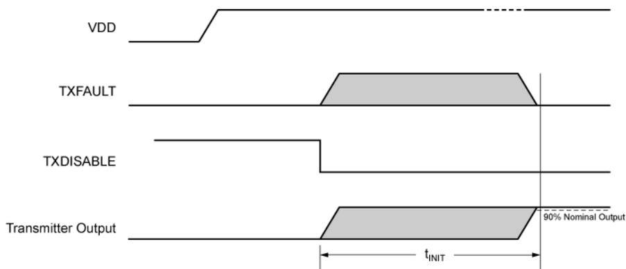
**Figure 16. Initialization Timing with TXDISABLE Not Asserted**
