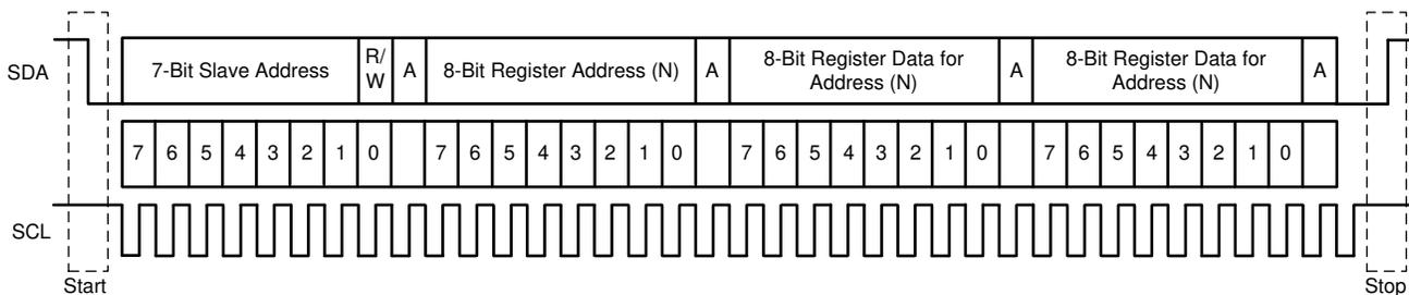
**Figure 9-9. Typical I<sup>2</sup>C Sequence**
