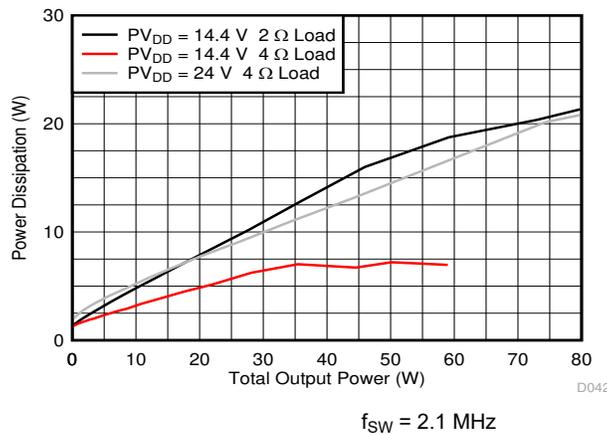
**Figure 7-33. BTL Power Dissipation vs Total Output Power**
