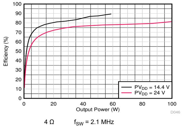
**Figure 7-16. Power Efficiency vs Total Output Power**
