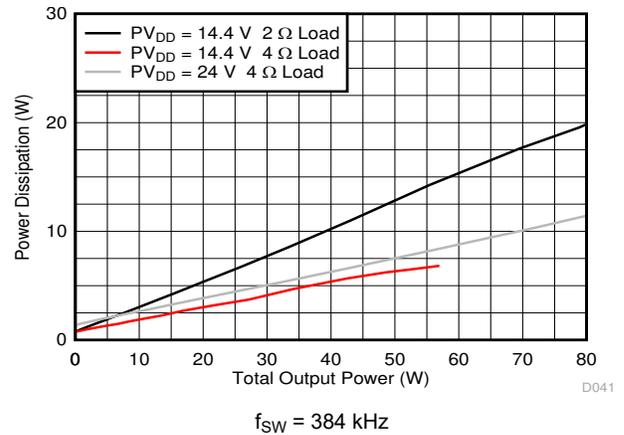
**Figure 7-32. BTL Power Dissipation vs Total Output Power**
