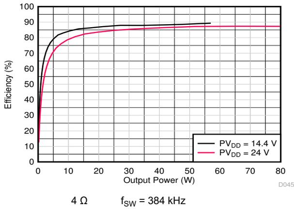
**Figure 7-15. Power Efficiency vs Total Output Power**
