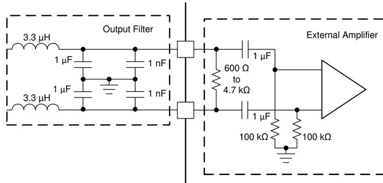
**Figure 10-1. External Amplifier Input Configuration for Line Driver**
