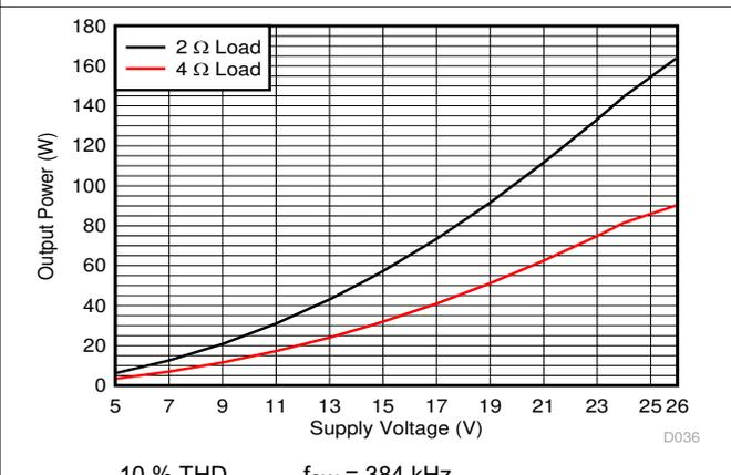
**Figure 7-30. PBTL Output Power vs Voltage**
