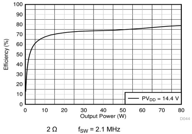
**Figure 7-18. Power Efficiency vs Total Output Power**
