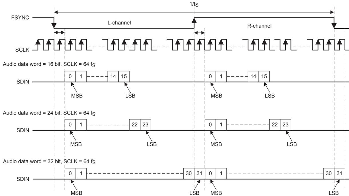
Figure 9-4. I<sup>2</sup>S Audio Data Format
