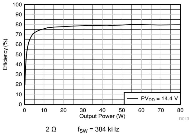
**Figure 7-17. Power Efficiency vs Total Output Power**
