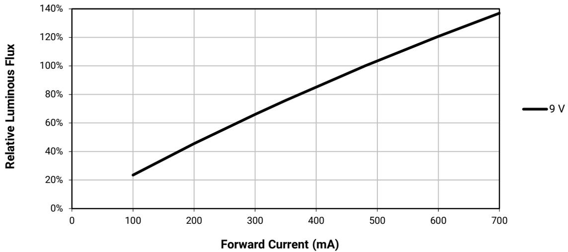
RELATIVE FLUX VS. CURRENT ( $T_j = 85\text{ }^\circ\text{C}$ ) - CONTINUED
