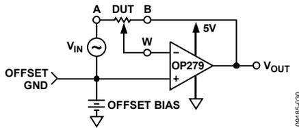
Figure 29. Inverting Gain
