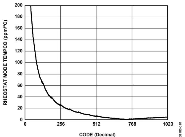
Figure 10.  $(\Delta R_{WB}/R_{WB})/\Delta T \times 10^6$  Rheostat Mode Tempco
