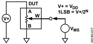
Figure 26. Potentiometer Divider Nonlinearity Error (INL, DNL)
