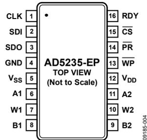
Figure 4. Pin Configuration
