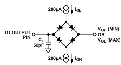
Figure 35. Load Circuit for Measuring V<sub>OH</sub> and V<sub>OL</sub> (The diode bridge test circuit is equivalent to the application circuit with R<sub>PULL-UP</sub> of 2.2 kΩ.)
