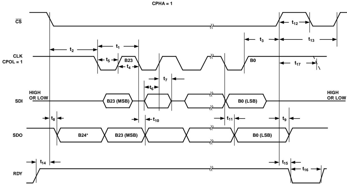
\*THE EXTRA BIT THAT IS NOT DEFINED IS NORMALLY THE LSB OF THE CHARACTER PREVIOUSLY TRANSMITTED. THE CPOL = 1 MICROCONTROLLER COMMAND ALIGNS THE INCOMING DATA TO THE POSITIVE EDGE OF THE CLOCK.
