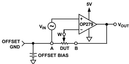
Figure 30. Noninverting Gain
