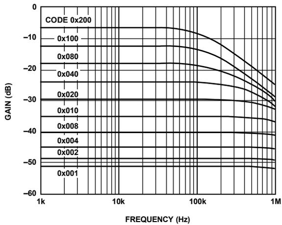
Figure 18. Gain vs. Frequency vs. Code (See Figure 31)
