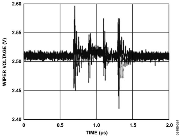
Figure 23. Digital Feedthrough
