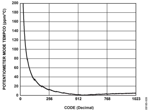
Figure 9.  $(\Delta V_w/V_w)/\Delta T \times 10^6$  Potentiometer Mode Tempco
