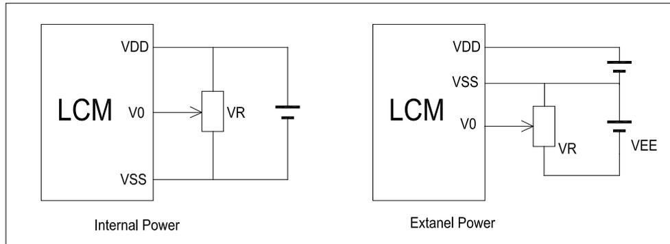
$V_{DD}-V_0$ : LCD Driving voltage
