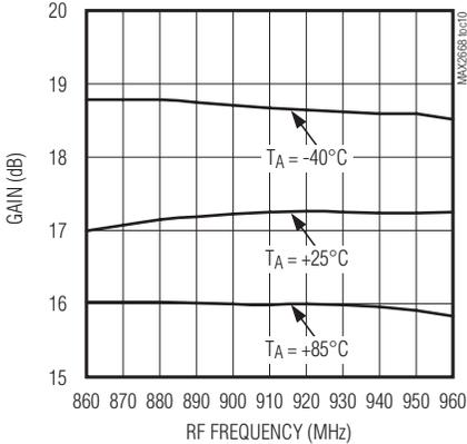
**MAX2668 GAIN vs. FREQUENCY AND TEMPERATURE MID-GAIN MODE**
