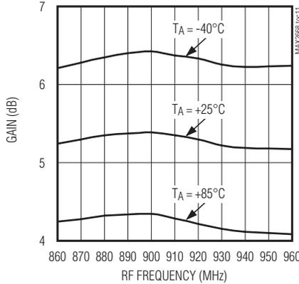
**MAX2668 GAIN vs. FREQUENCY AND TEMPERATURE LOW-GAIN MODE**
