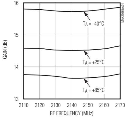
**MAX2666 GAIN vs. FREQUENCY AND TEMPERATURE MID-GAIN MODE**
