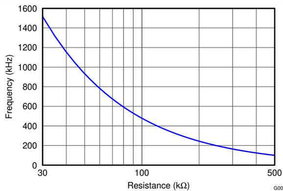
**Figure 6-5. Frequency vs FREQ Resistance**
