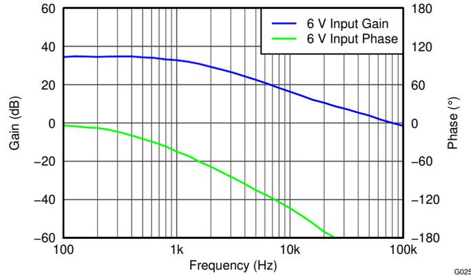
**Figure 8-11. SEPIC Power Stage Gain and Phase**
