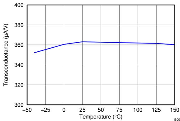
**Figure 6-1. Error Amplifier Transconductance vs Temperature**
