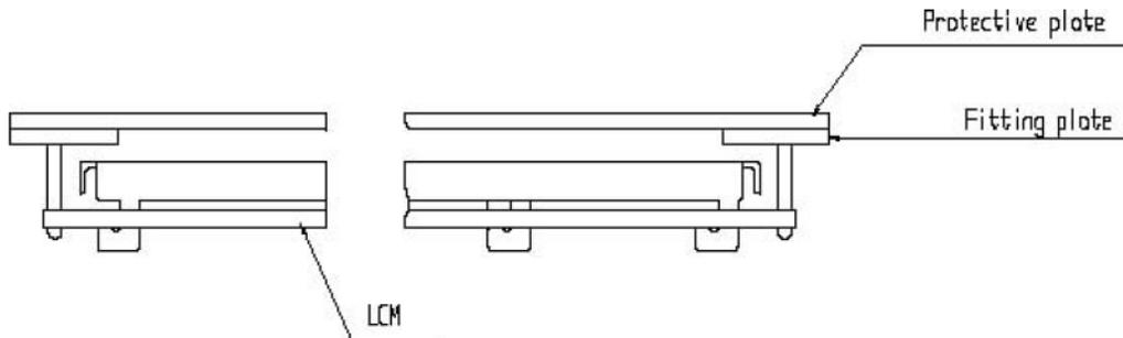
2. When assembling the LCM into other equipment, the spacer to the bit between the LCM and the fitting plate should have enough height to avoid causing stress to the module surface, refer to the individual specifications for measurements. The measurement tolerance should be  $\pm 0.1\text{mm}$ . Precaution for assemble the module with BTB connector:
