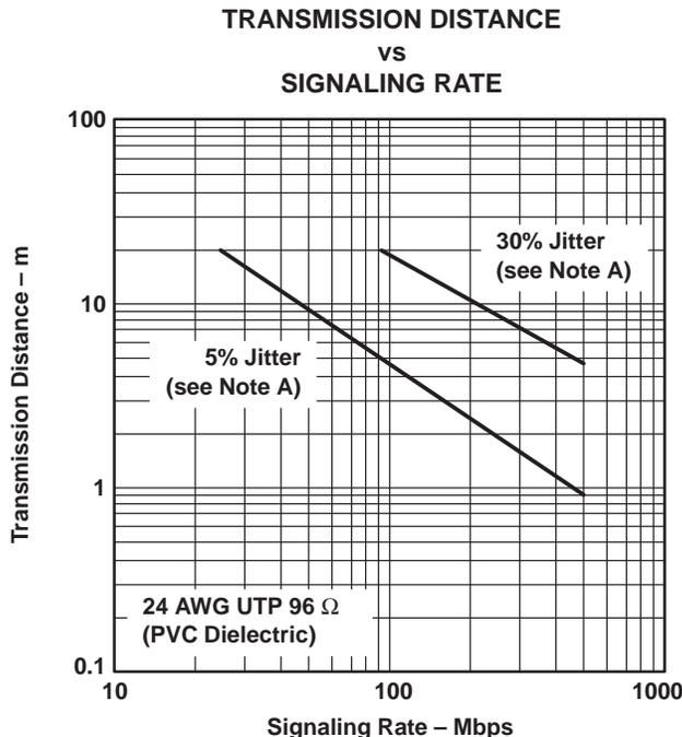
NOTE A: This parameter is the percentage of distortion of the unit interval (UI) with a pseudorandom data pattern.
