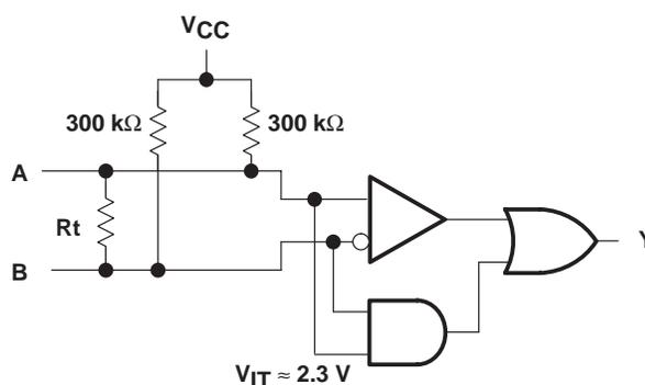
Figure 9. Open-Circuit Fail Safe of the LVDS Receiver
