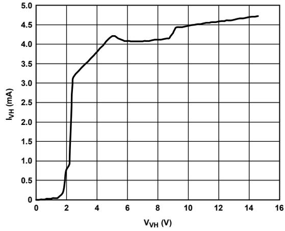
Figure 8.  $I_{VH}$  vs.  $V_{VH}$  (VH as Supply)
