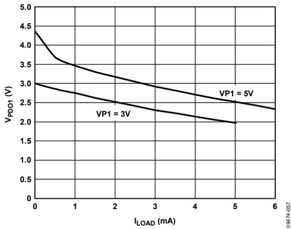
Figure 11.  $V_{PDO1}$  (Strong Pull-Up to  $VPx$ ) vs.  $I_{LOAD}$
