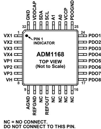
Figure 3. Pin Configuration
