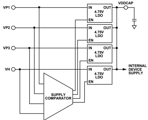
Figure 14. V<sub>DD</sub> Arbitrator Operation
