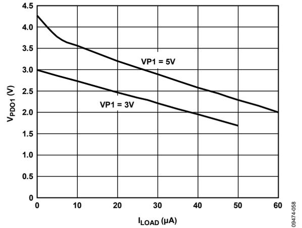
Figure 12.  $V_{PDO1}$  (Weak Pull-Up to  $VPx$ ) vs.  $I_{LOAD}$
