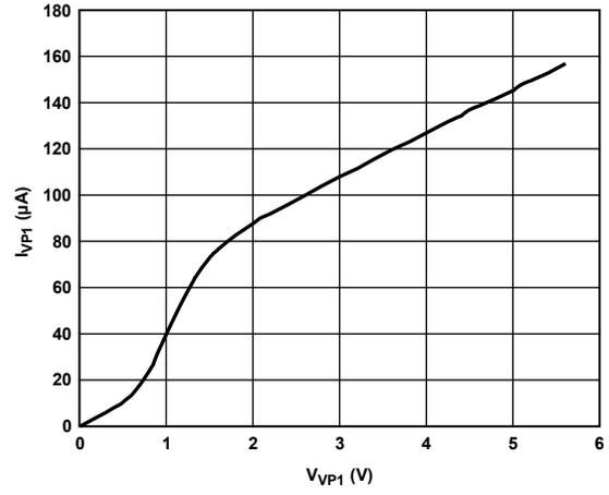
Figure 7.  $I_{VP1}$  vs.  $V_{VP1}$  (VP1 Not as Supply)
