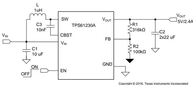
The typical operating frequency is 1.15 MHz, which allows the use of small inductor and capacitors to achieve a small solution size. The TPS61230A provides an adjustable output voltage via an external resistor divider.
