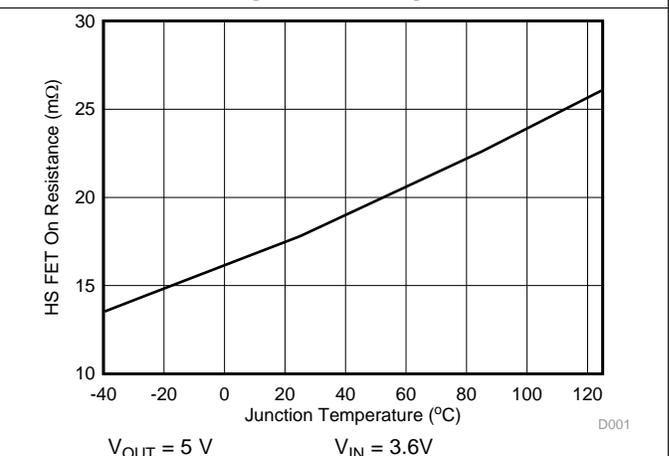
Figure 6. High-Side FET  $R_{ds(on)}$  vs. Junction Temperature
