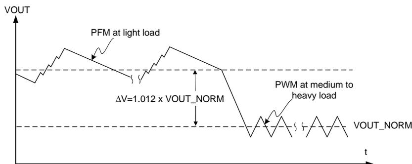
**Figure 14. Output Voltage in PFM / PWM Mode**
