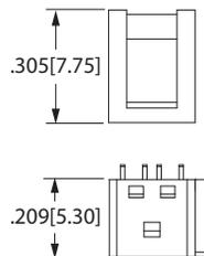
**INSULATION DISPLACEMENT (ID) without Strain Relief**
