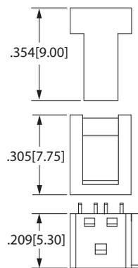
**INSULATION DISPLACEMENT (ID) with Strain Relief**
